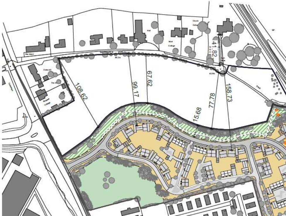
Figure 5.1: Key dimensions (in meters) between the proposed development and The Forest/St Mary's Church
