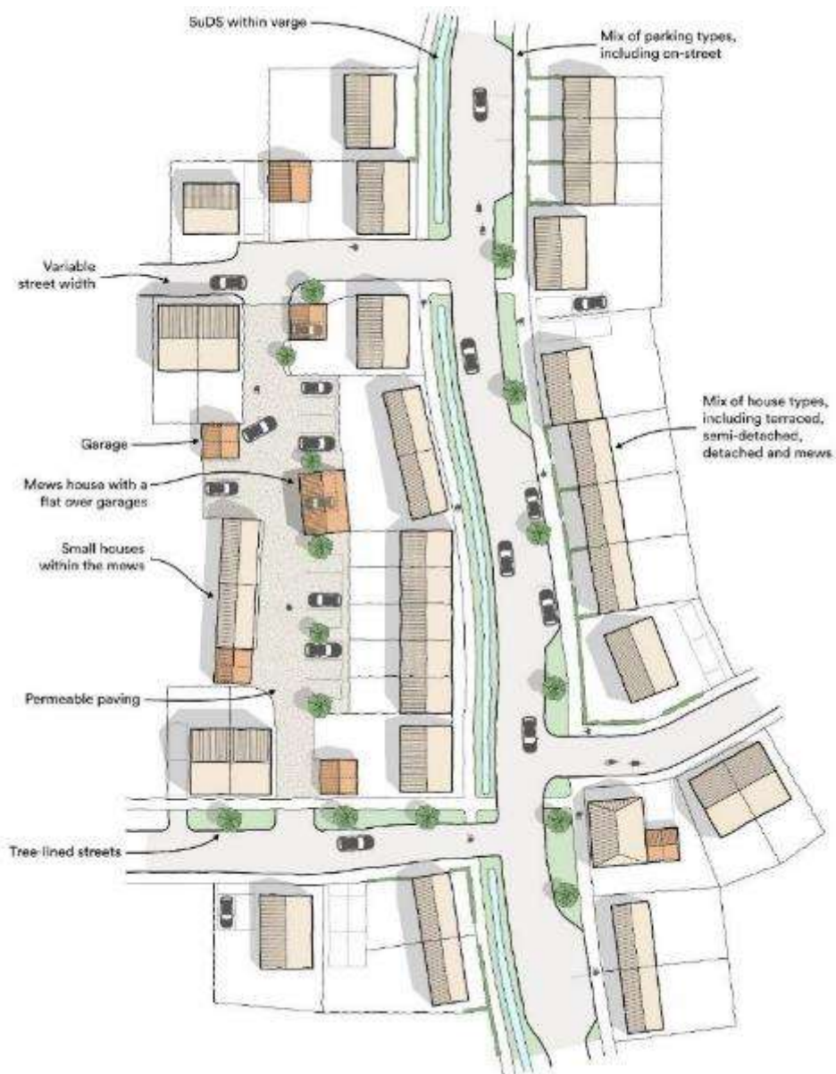
An example of a secondary street with a mews behind and a network of local and tertiary streets branching off
