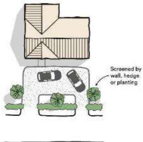
Front courtyard parking can be used with larger homes with a separate entrance and exit
