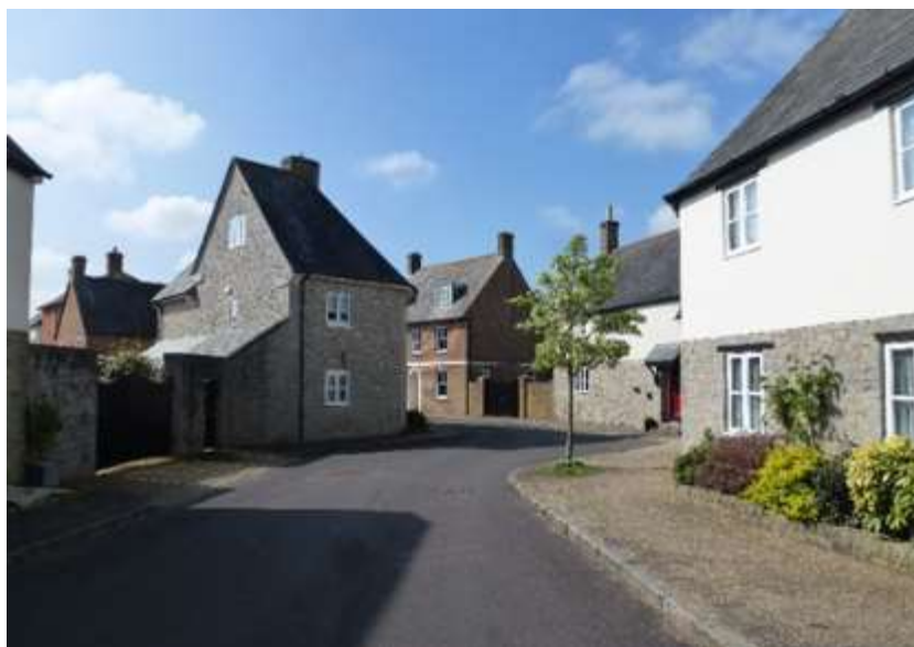
Carriageway deflection, sharp corner radii, street trees and changes in material all help reduce speeds in residential streets in Poundbury (image credit Andy Cameron)
