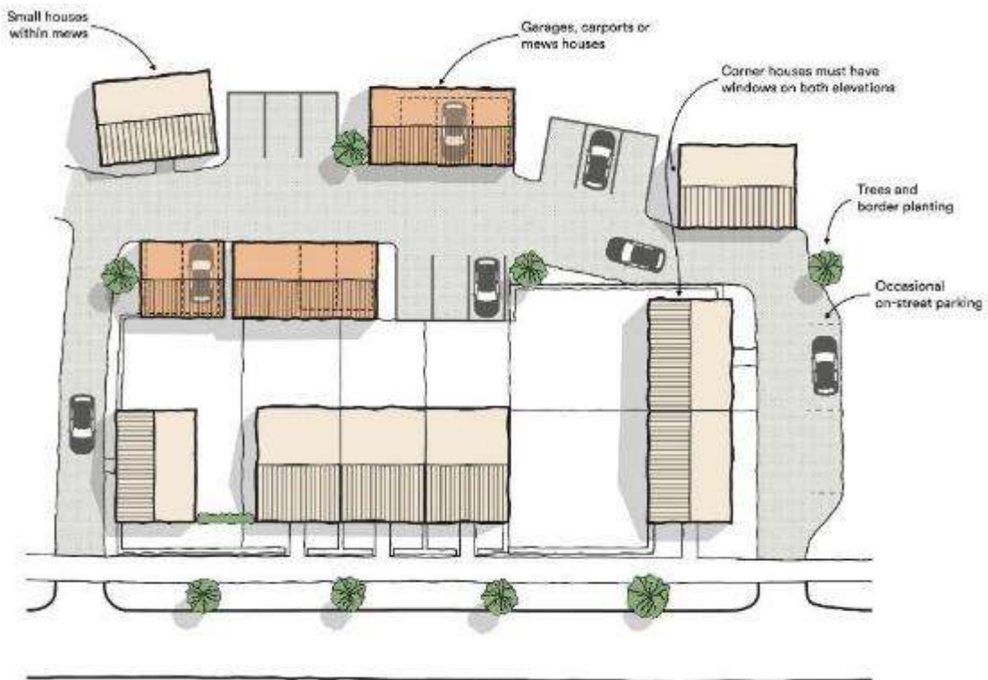
Formal mews parking for a town centre, local centre or suburban development
