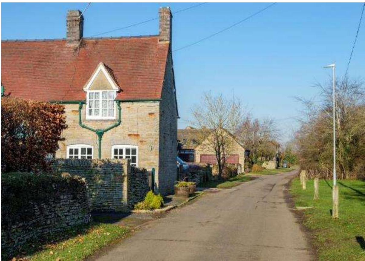
On streets without kerbs, such as this street in North Littleton, verges can play an important role in absorbing rain runoff without the need for extensive infrastructure
