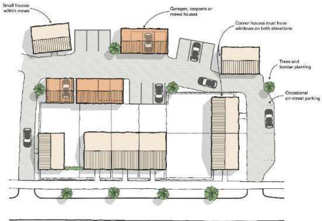
Formal mews parking for a town centre, local centre or suburban development
