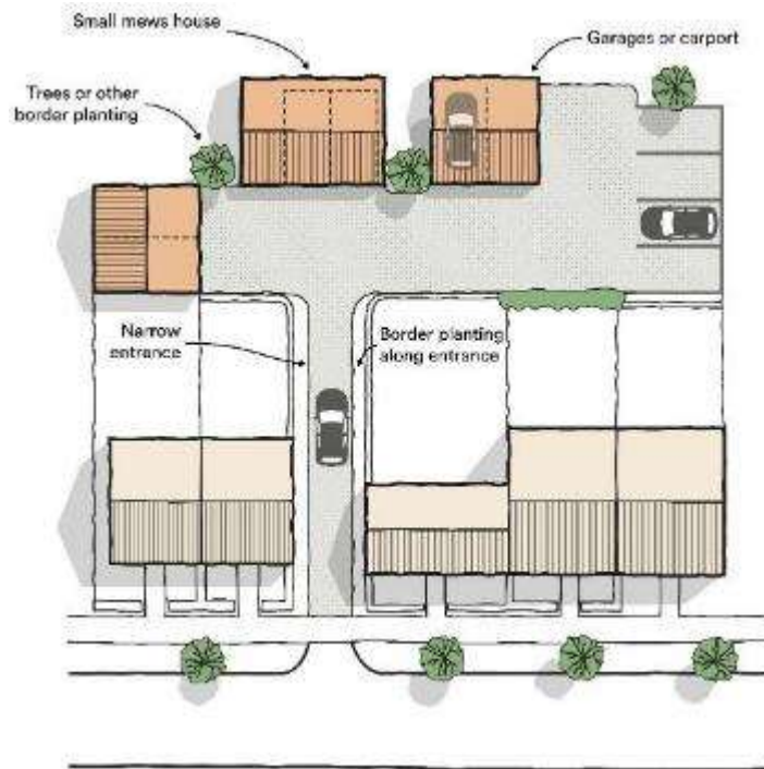
Formal rear parking for a town centre, local centre or suburban development
