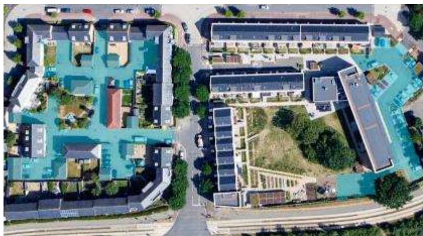
The development to the left uses a combination of courtyard, on-street and curtilage parking. The development on the right uses peripheral parking at the edge of the site. As a result, the development on the left uses roughly seven times as much land for car access and storage whilst creating a far lower quality of public realm
