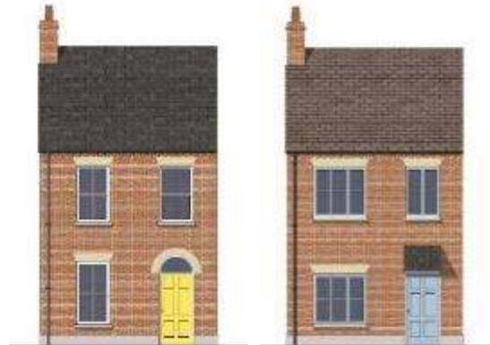
2 storey narrow house Should be built in a terrace or semi-detached Pictured with sash and casement window options
