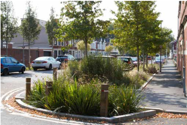
Street 'rain gardens' and conveyancing rills/drains
